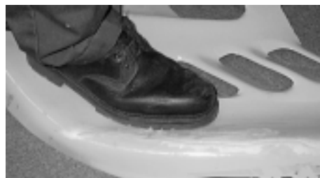
Repairs made to Ski-Doo PUR cowls with 5003R1 urethane rod are tough.
