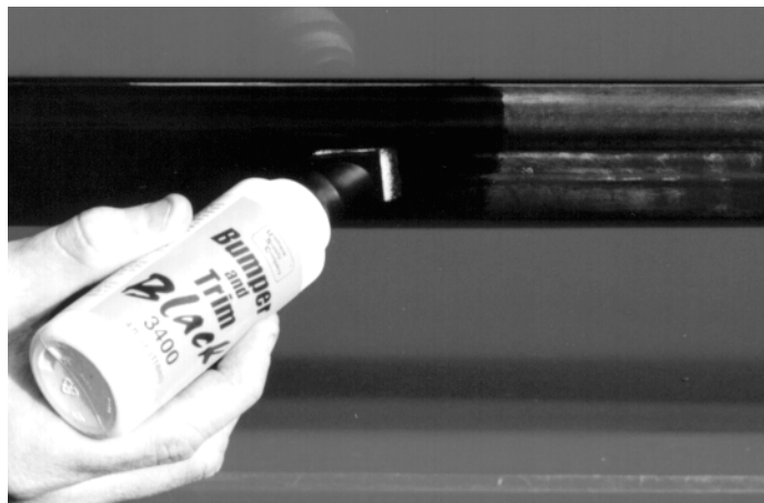
Applying the Bumper and Trim Black over wax-stained side trim is a breeze with the built-in applicator
